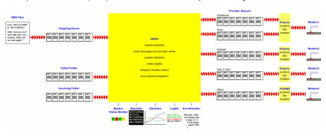
The picture shows how the SMS Server Tools send SM. In this case we have five british phone network provider and we use four modems to send messages.
