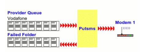
Any provider queue as at least one attached modem. One program part of smsd (modem task) reads the SMS files from the provider queue and sends it using the sub-program putsms.
