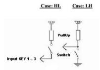
The alarm inputs work only, when the modem gets power from an external power supply. The internal battery does not source this part of the modem with energy.
