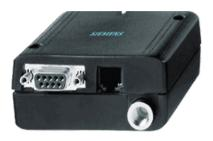
The Siemens TC35 terminal is the actual widely used GSM modem from Siemens.
