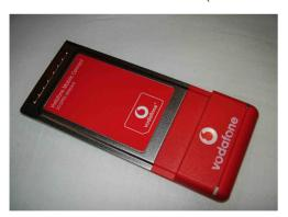
This Modem card has got an internal USB Controller and a USB2Serial adapter. The modem inside this card is a serial modem. This card can be used under Linux by loading the driver with the following commands:
