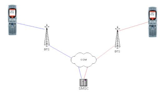
The short message is normally entered via the keypad of the mobile phone and stored onto the SIM card. Then is is sent through the signalling channel to the SMSC. This channel is also used for call setup.
